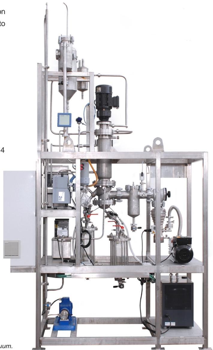
*Pilot plant distillation under high vacuum.*
